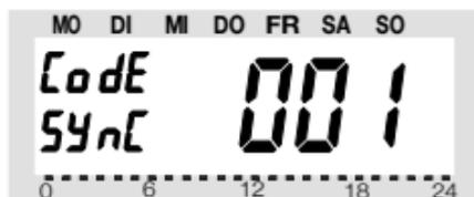
Now you have to synchronise the (first) valve operating mechanism (“001” on the display) to the new safety code.
